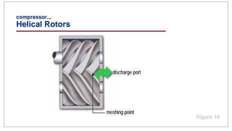
Finally, when the pockets of refrigerant reach the **discharge port** the compressed vapor is released. As the rotors continue to rotate, the volume of the pockets is further reduced, squeezing the remaining refrigerant from the cavities.
